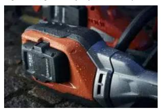
Weatherproof (IPX4) – This battery-powered Husqvarna machine fulfils the IPX4 classification for rain resistance. This makes it a long-lasting and reliable tool that can be used all year round in all weather conditions.
