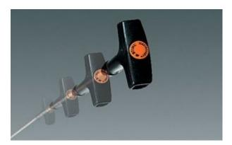
Stihl Elastostart - STIHL ElastoStart reduces the shock caused by the compression of the engine during starting. The compression shock is taken away from the user's joints and muscles through a spring or rubber element in the starter handle.
