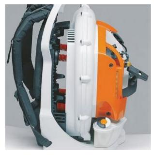
Anti-Vibration System - Intense vibration at the handles of power tools can lead to long-term effects on blood vessels in the hands and arms. STIHL has therefore developed an effective anti-vibration system whereby the oscillations from the machine's engine are dampened which significantly reduces vibrations at the handles.
