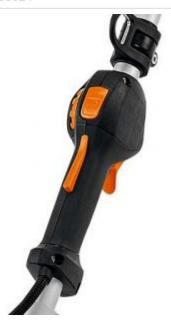
Stihl Ecospeed – With the ECOSPEED function, you can use your long reach hedge trimmer in a more economical operating mode. Simply turn the wheel to the minus direction, thereby reducing the maximum engine speed. This keeps your long reach hedge trimmer running at partial load; however, despite this limited setting, you can shift to full capacity when necessary by pressing the throttle lever. Operating at partial load reduces fuel consumption and you can work much longer with one tank.
