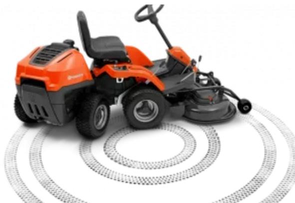
**Articulated Steering** - The articulated steering gives excellent manoeuvrability and facilitates driving around obstacles such as trees and bushes.
