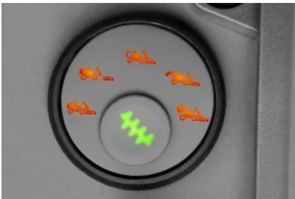
Non-collecting mode - Easy switch between collecting and non-collecting mode by just pushing a button. You don't have to leave the driver's seat.
