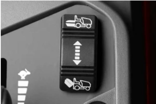
Empty collector from the seat - The integrated collector is easily emptied from the driver's seat
